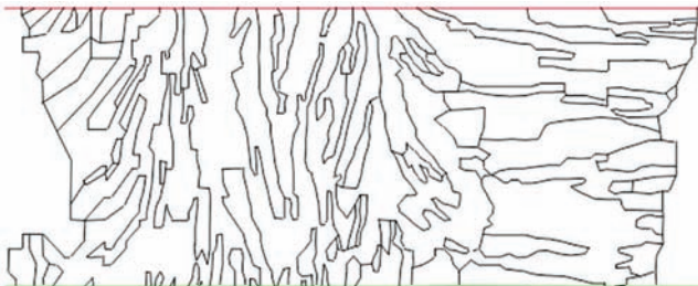
Figure 4. The CAD drawing of the zone 1 weld cross-section input into the CIVA model. The drawing consists of 89 closed regions with a total of 1276 boundaries
