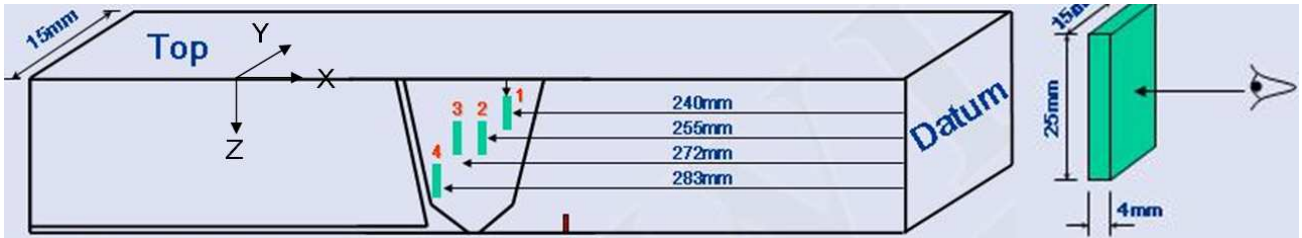
Figure 7 Positions of samples extracted from the weld for length measure of grains in y direction.
